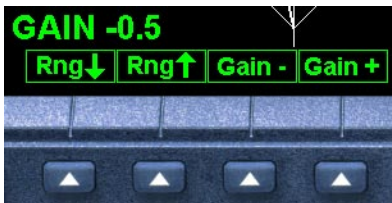
Radar Gain Control
