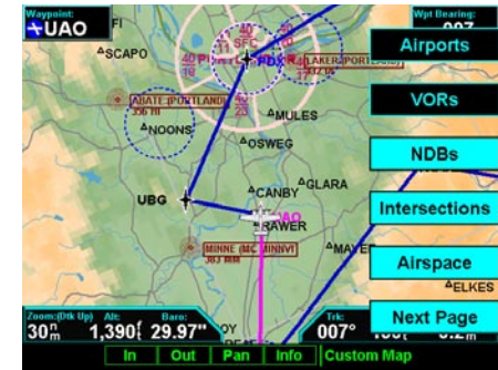
Custom Map page with NDBs, Intersections, and Airspace selected with Menu Items (Page 2)
